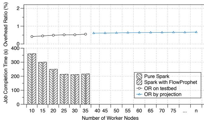
Fig. 15: FLOWPROPHET scalability evaluation on WikipediaPageRank-26G (Spark).
